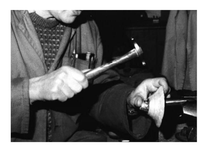
After annealing, the shaping of the foot and the cup can be taken to a further stage by hammering on a suitably shaped stake held in a vice. This is called 'raising'.
