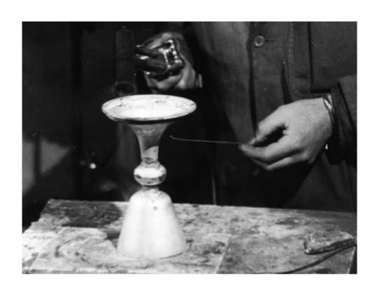
Using the centre point of the original blank, a circle is drawn onto the bottom of the cup to mark the position of the base and then the base and the cup are soldered together.
