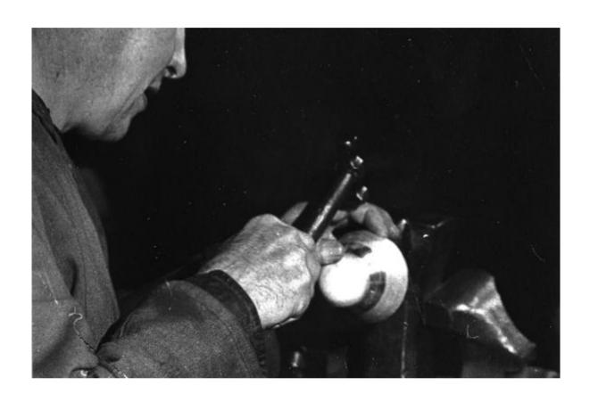
Once the basic shape is achieved through raising, the surface is very rough and bumpy. The surface is then smoothed by hammering the silver with a lighter hammer over a stake that matches the shape perfectly giving an appearance which is characteristic of handraised silverware. This is called 'planishing'.
