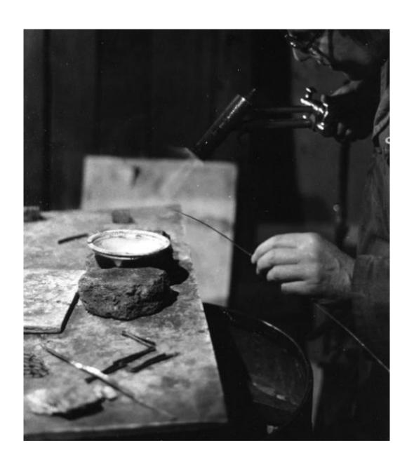
All the parts are joined together by heating and melting a stick of solder into the joints to create one whole piece. This is called 'soldering'.
