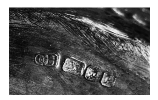
A sample of the metal is scraped from the surface and analysed. It must contain not less than 92.5% of pure silver before receiving the hallmark.
