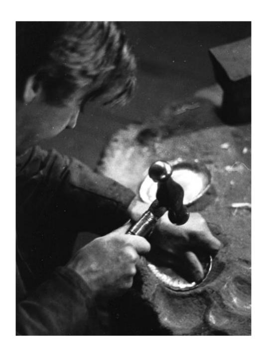
There is a large tree stump in the middle of the workshop with depressions carved into its surface in which the first shaping operation is done. This is called 'blocking'.
