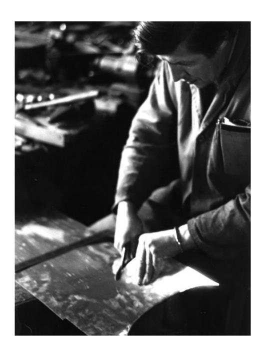
The blanks for the cup, the foot and the knop are drawn and then cut from the sheet of silver. The centre point is kept for subsequent operations.
