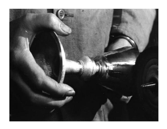
The final operation is polishing with an electricallydriven motor on which polishing mops and brushes are fitted.
